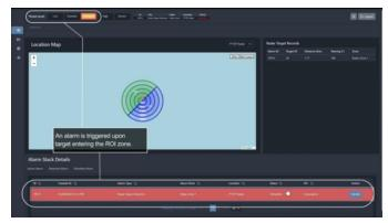
Alarm Trigger: An alarm is immediately triggered when a target or intruder enters the predefined Region of Interest (ROI) zone, allowing for prompt response.
