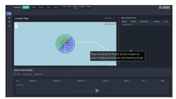
UI Visualization: The Simpnify platform provides an intuitive user interface that displays a radar map with user-configured zones based on distance and bearing range. This helps in monitoring specific areas effectively.
